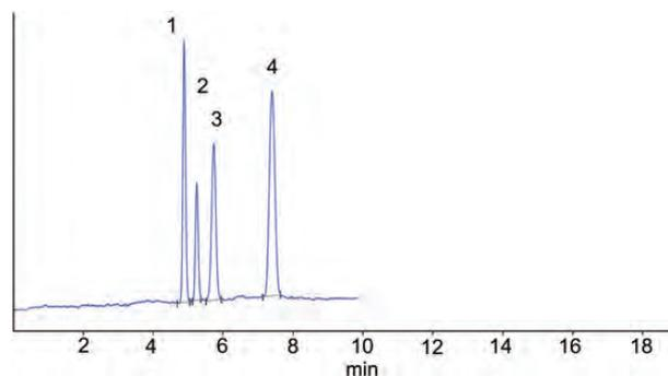
**Figure 3.** Chromatogram in cLC with the monolithic column. Conditions were as described in the following. Column: monolithic poly(SPE-co-PETA), 250 mm (total length 500 mm)  $\times$  100  $\mu$ m i.d.; mobile phase, ACN–H<sub>2</sub>O (93/7, v/v) containing 50 mmol/L ammonium formate; pump flow rate, 0.05 mL/min; backpressure, 1.5 MPa; detection, UV at 214 nm. Samples: toluene (1), paracresol (2), paranitrophenol (3), hydroquinone (4).
