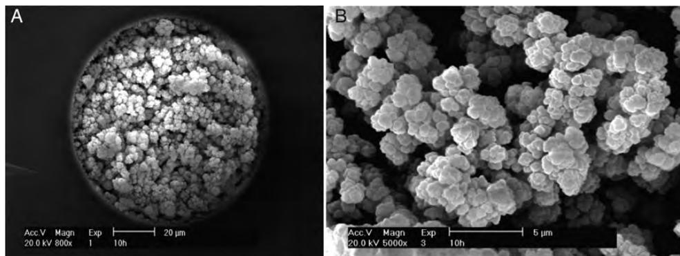
**Figure 1.** Scanning electron micrographs of the monolithic columns.
