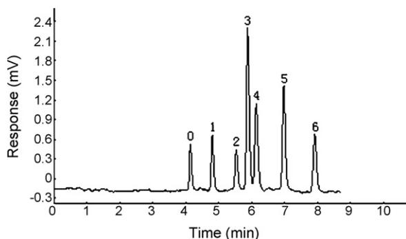
**Fig. 6.** Electrochromatogram of phenols. Capillary column, column C; experimental conditions: mobile phase, 5 mmol/L TEAP buffer; other conditions as in Fig. 5. Solutes: (0) toluene, (1) phenol, (2) catechol, (3) resorcinol, (4) hydroquinone, (5) pyrogallol, (6) phloroglucinol.
