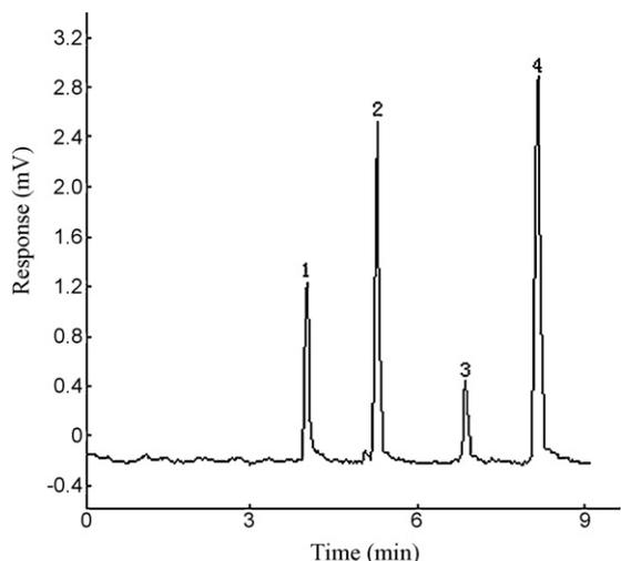
**Fig. 7.** Electrochromatogram of some model compounds. Capillary column, column C; experimental conditions as in Fig. 6. Solutes: (1) toluene, (2) DMF, (3) formamide, (4) thiourea.
