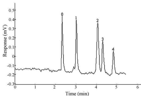
**Fig. 8.** Electrochromatogram of amides. Capillary column, column C; experimental conditions: mobile phase, TEAP buffer in ACN/H<sub>2</sub>O (98/2, v/v); other conditions as in Fig. 6. Solutes: (0) toluene, (1) DMF, (2) *N,N*-dimethylenbisacrylamide, (3) formamide, (4) acetamide.
