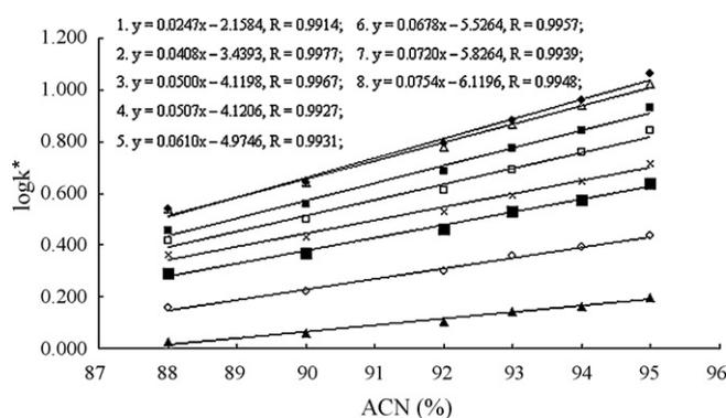
**Fig. 10.** Plots of  $\log k^*$  for nucleic acid bases and nucleosides versus percent ACN (v/v) in the mobile phase. Capillary column, column C; experimental conditions: mobile phase: TEAP buffer in ACN/H<sub>2</sub>O (v/v); other conditions as in Fig. 6. Lines: (1) uracil, (2) uridine, (3) adenosine, (4) adenine, (5) cytosine, (6) cytidine, (7) guanine, (8) guanosine.
