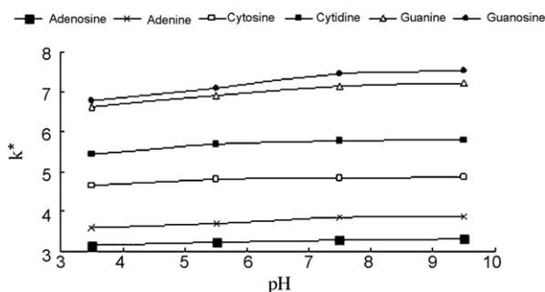
**Fig. 11.** Effect of pH on the retention factor ( $k^*$ ). Capillary column, column C; experimental conditions: mobile phase: TEAP buffer in ACN/H<sub>2</sub>O (93/7, v/v); other conditions as in Fig. 6.
