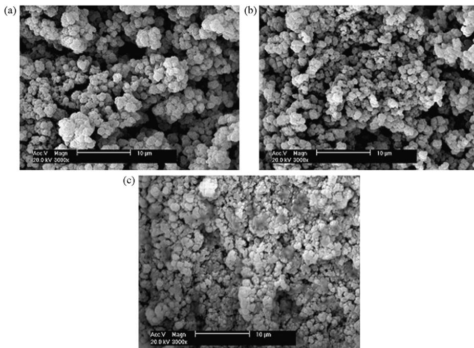
**Fig. 2.** Scanning electron microphotographs of monolithic columns prepared with different dodecanol weight fraction: (a) column B; (b) column C; (c) column D.
