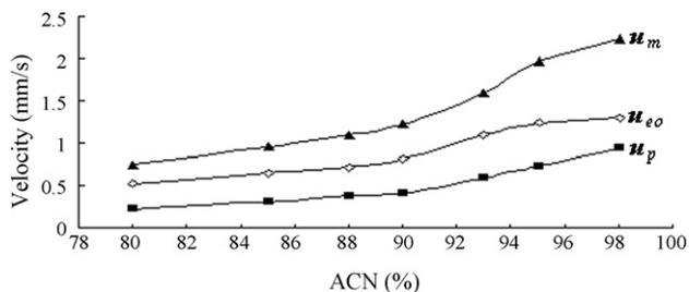
Fig. 4. Effect of ACN content on the EOF,  $u_p$  and  $u_m$ . Capillary column, column C; experimental conditions: mobile phase,  $5 \text{ mmol/L}$  TEAP buffer pH 8.5 in ACN/ $\text{H}_2\text{O}$  (90/10, v/v); applied voltage:  $-20 \text{ kV}$ ; other conditions as in Fig. 1.
