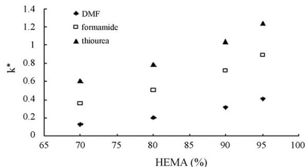
Fig. 3. Plots of retention factors ( $k^*$ ) versus HEMA (wt%) in the monomer mixture. Experimental conditions: applied voltage:  $-20 \text{ kV}$ ; other conditions as in Fig. 1.
